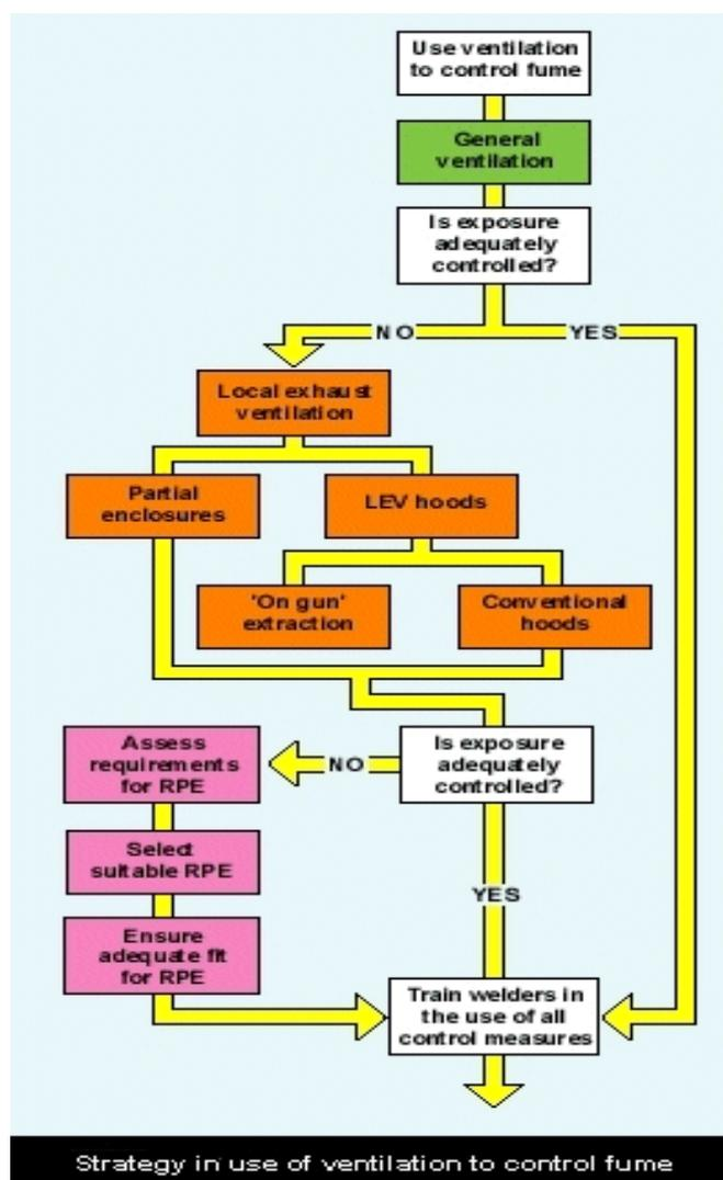
Figure 4 Controlling welding fume. [TWI Ltd.]
