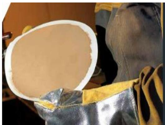
**Figure 1** Filter paper with particulate welding fume.
