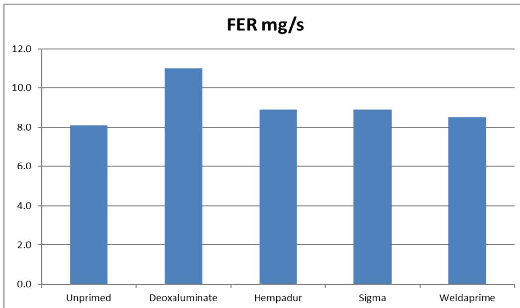
**Figure 2** Fume emission rate results in mg/s.
